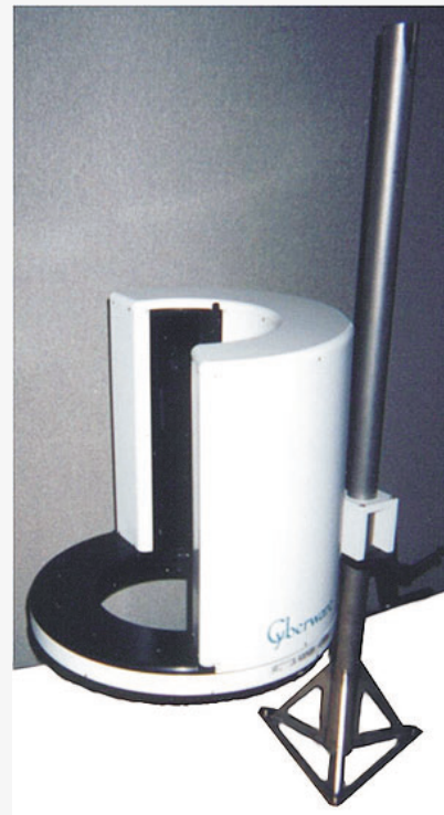
The Below the Knee (BK) custom 3D scanning system was designed to digitize the residual limb of a below knee amputee.
